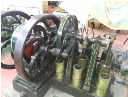
The "Clutterbuck Bros" engine (left) had spare sleeves standing by for quick reconditioning.
